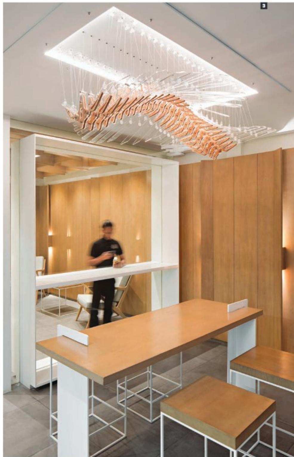
Above the coffee bar, a kinetic installation represents the crow of Kisaku logo and brings a slow and hypnotizing dynamism into the room. It is composed of 25 moveable bone-shape wood frames and thin acrylic wings, hanging from the ceiling with thin wires. The steel wires are connected to individually controllable motors that arise and lower the ends of each lamella, allowing various "flying" movement patterns to be performed.
